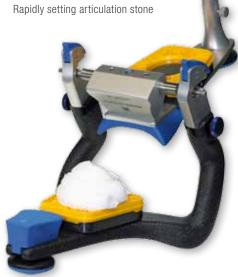
To fix working models in the articulator and position relinings. Artigips is also suitable for orthodontic work. Artigips convinces with its precision and low setting expansion (< 0.08%).
