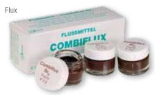
Combiflux-Paste (BrP) is a special flux for soldering non-precious and precious metal alloys as well as non-precious to precious metal alloys. Combiflux-Paste (BrP) removes surface oxides completely. Combiflux products do not blow out and burn out completely. Combiflux is very active and should therefore only be used in small quantities.
